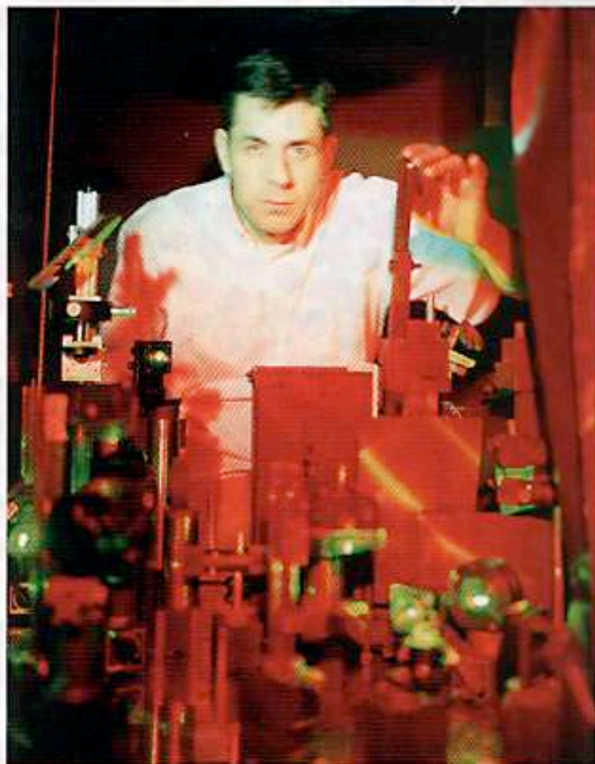
Yves Gentet adjusts an optical bench in his lab in Bordeaux, France. The bench holds some 120 optical instruments used in the making of Gentet's most complex multichannel holograms.
